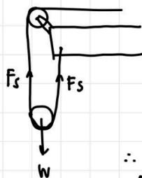
∴ The input torque required from the motor is 4.95 oz-in and the corresponding RPM is 56.58 RPM (14.1458 RPM for a 4:1 gear ratio). The predicted time to lift the 10-lb weight is 5.4 seconds.
