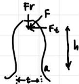
Find: the maximum bending stress at the root of a gear tooth
