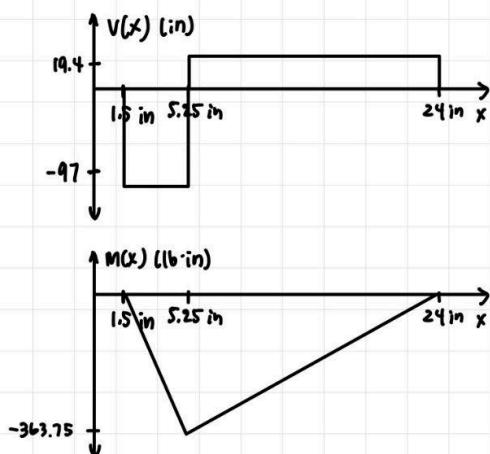
$$\sigma_{\max} = -\frac{M_{\max} y}{I} \quad I = \frac{1}{12} b h^3 = \frac{1}{12} (0.5 \text{ in})(2 \text{ in})^3 = 0.33 \text{ in}^4$$
